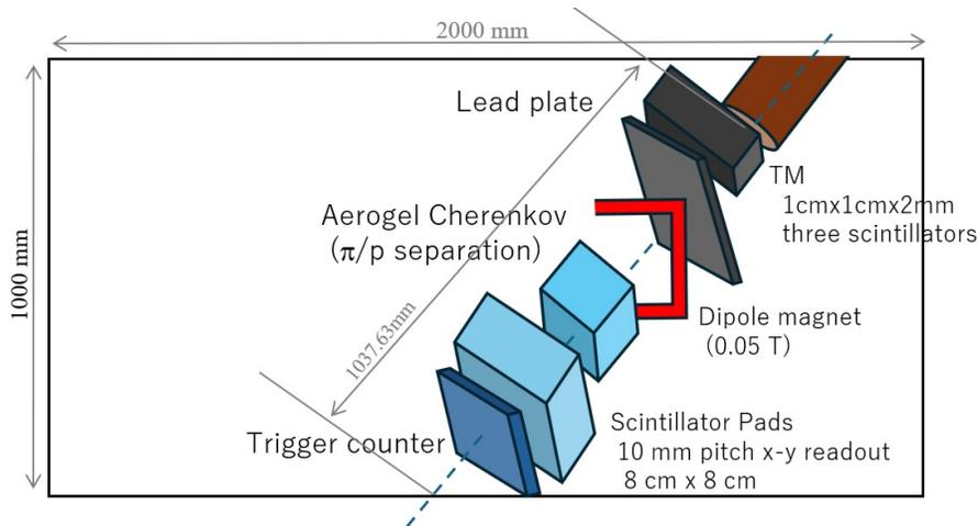
Figure 4: Expected setup to measure charged pion rate at the hadron test beam line in the K1.8 BR area.
