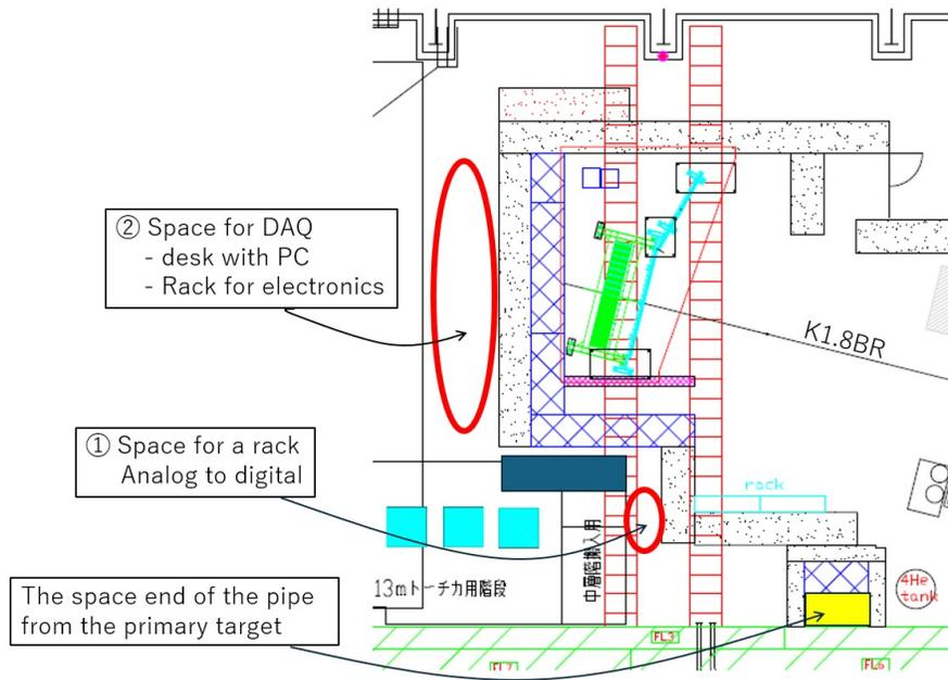
Figure 5: Location of readout DAQ at the hadron test beam line in the K1.8 BR area. It's good to have a rack close to the space to set module for analog signal treatment and discriminators. Rest of DAQ system will be placed on the behind of K1.8 BR line.
