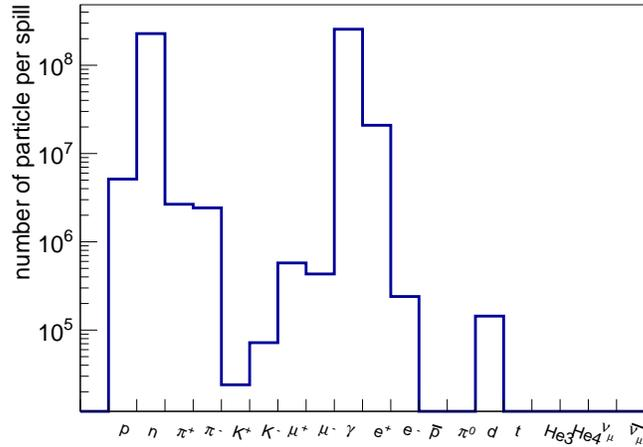
Figure 2: Expected distribution of particle species at the hadron test beam line in the K1.8 BR area (by the MARS simulation). Scale of y-axis is number of particle per spill at 115 kW operation.
