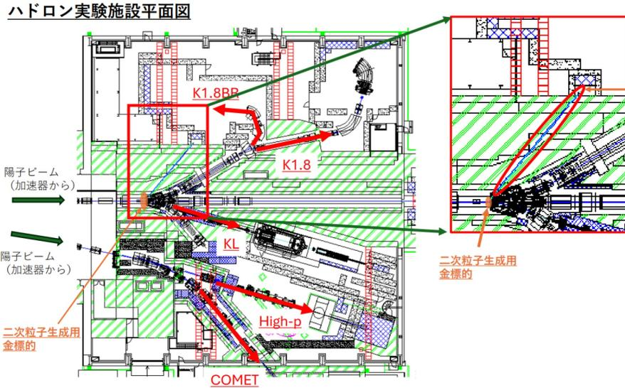
Figure 1: Floor map of the hadron hall. The zoom up box on the right shows the pipe location from the primary target to the test beam line.
