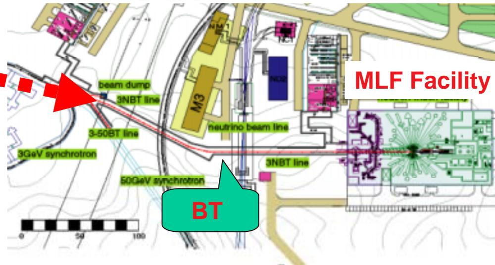
Beam dump is placed **underground** of the proton beam transport(BT) line.
