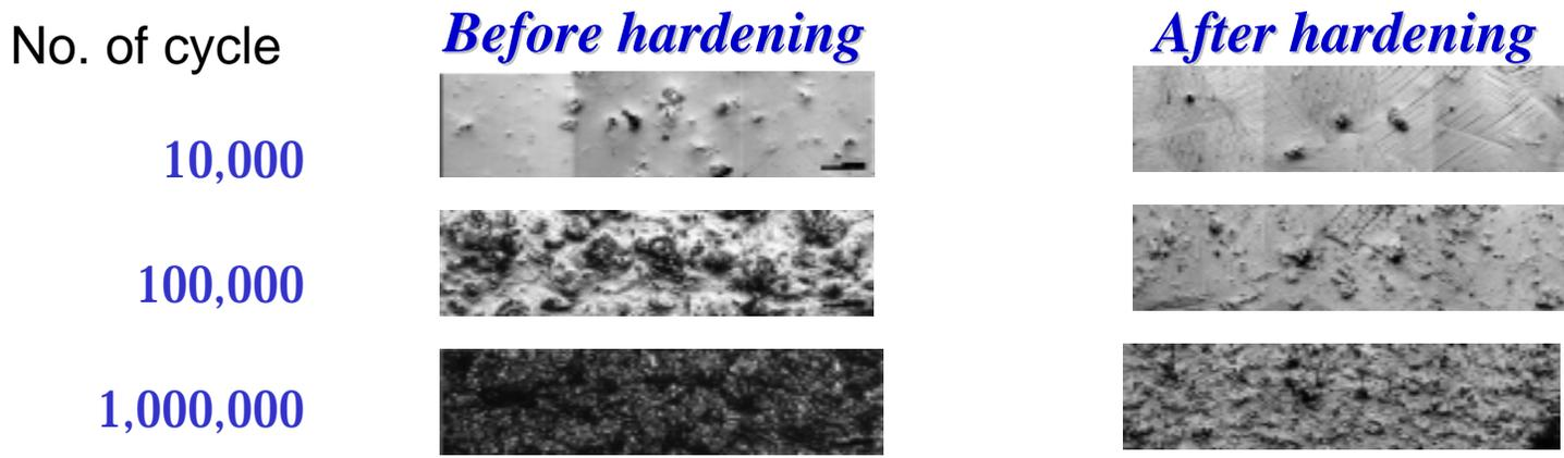
It is clearly observed that the pitting damage is suppressed by the hadning
