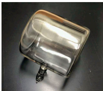
Figure 1. ^3\text{He} spin filter fabricated at J-PARC.
