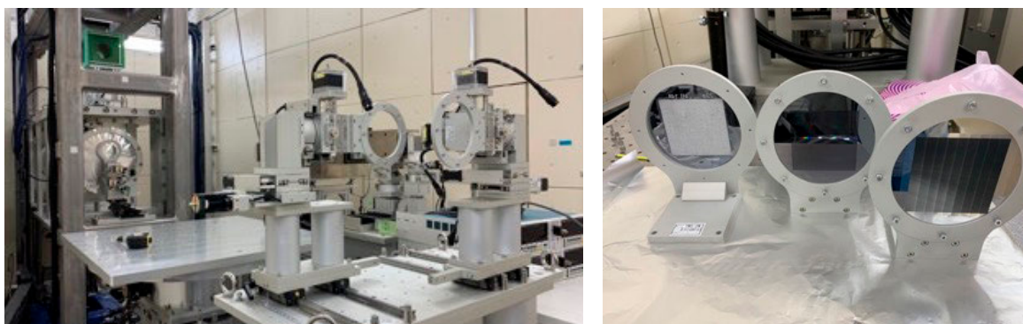
Figure 2. Photographs of the new phase imaging apparatus. Left: neutron Talbot-Lau interferometer installed at RADEN. Right: newly fabricated gratings.
