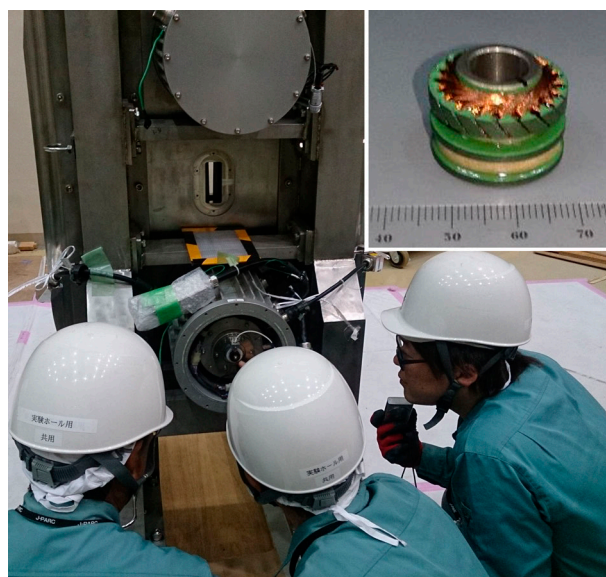
Figure 1. The monochromating disk-chopper under inspection. Inset shows a failed resolver.
