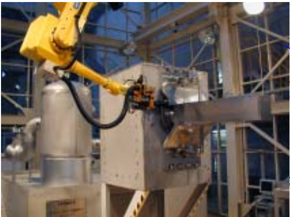
Remote-handling tests using an overhead traveling power manipulator
