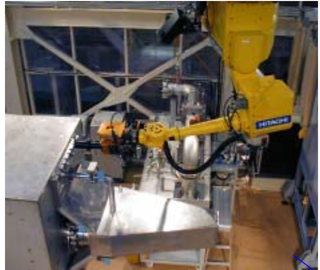
Remote-handling tests using an overhead traveling power manipulator
