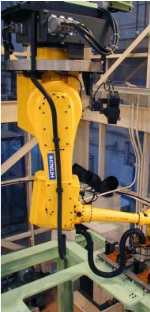
Automatic Exchange of End-effector
