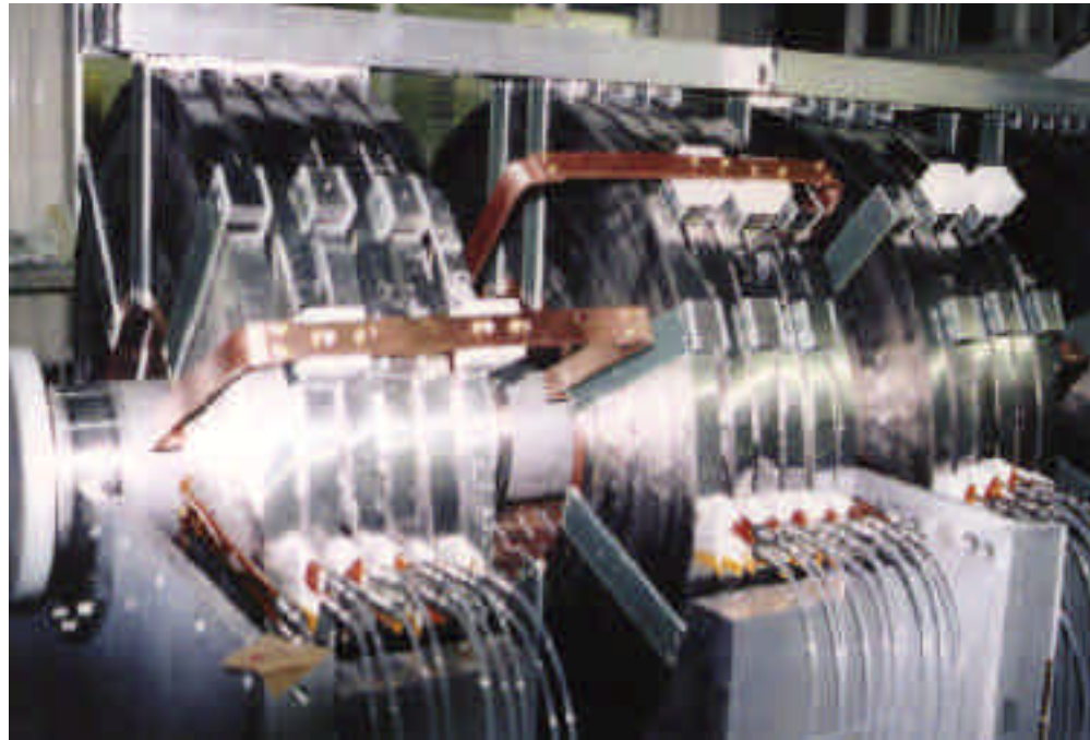
FINEMET-loaded Accelerating RF Cavity
