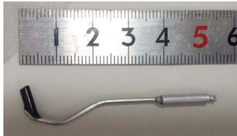
Fig. 1: Single crystal for the neutron diffraction measurement on BL-18.
