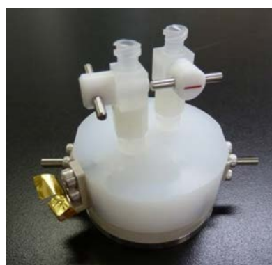
Figure 2 Electrochemical cell for neutron reflectometry.
