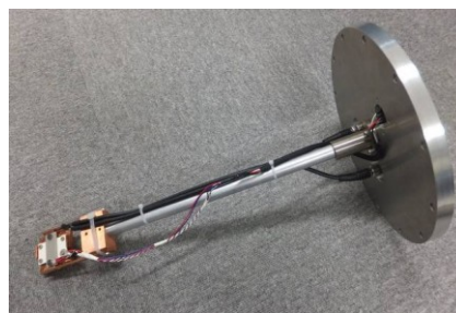
Fig. 2 A special sample holder for the spin-Seebeck effect measurements in the pole piece of the electromagnet of BL17.
