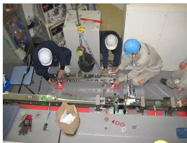
Figure 4. Re-alignment of AMATERAS beam-transport.
