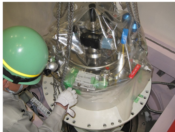
Figure 3. A BL-common 7T cryomagnet on AMATERAS.
