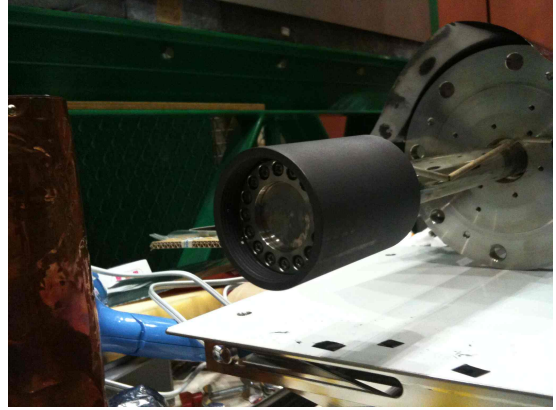
Fig.1 An improved oven for the \text{MgH}_2 measurements. Thanks to this oven, we obtained the change in a dynamic behavior of “milled with \text{Nb}_2\text{O}_5 sample” during the H-desorption reaction.
