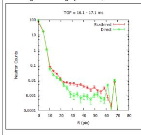
Fig.2 Profiles of beams measured with the sample (red) and without it (green) as a function of distance from the beam center. The difference in neutron counts corresponds to small angle scattering by the sample ( $Fe_{99.35}Cu_{0.65}$ ). Size of the detector pixel is 0.33 mm.
