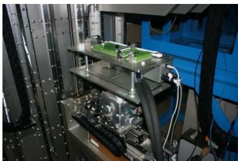
Fig. 1 The Langmuir-Blodgett trough used in the in-situ neutron reflectivity study to prepare monolayer at the air- D_2O interface.
