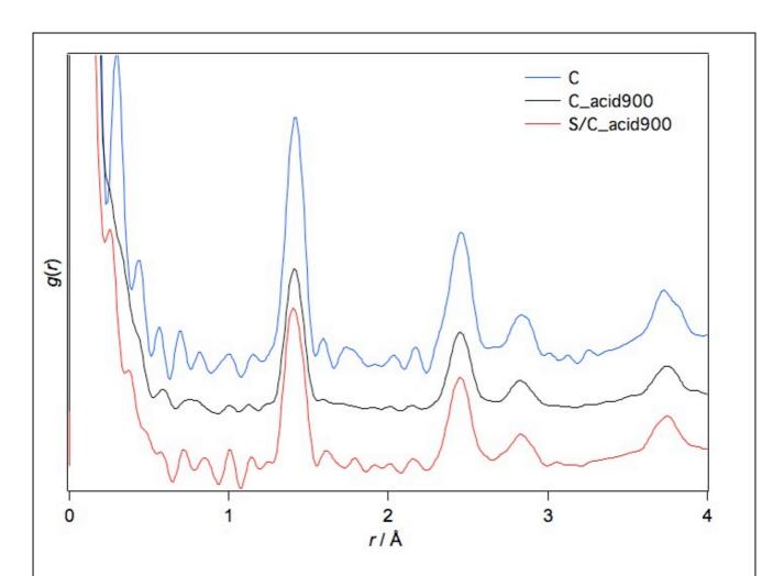
Fig. 1 pair distribution function, g(r), for Carbon nanotube and sulfur/carbon nanotube composite material.
