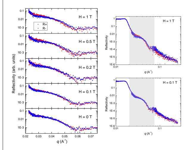
The detailed analysis of the PNR data is now underway, and by combining with the X-ray magnetic circular dichroism data, the magnetic structure of Ni at the interface to antiferromagnetic FeMn will be revealed. To the best of our knowledge, this is the first time to apply PNR to such thin films without a multilayer structure.
