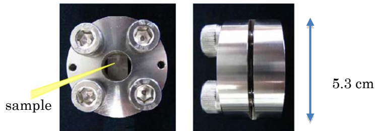
Fig. 1 Sample folder for measuring SANS under stress and magnetic field
