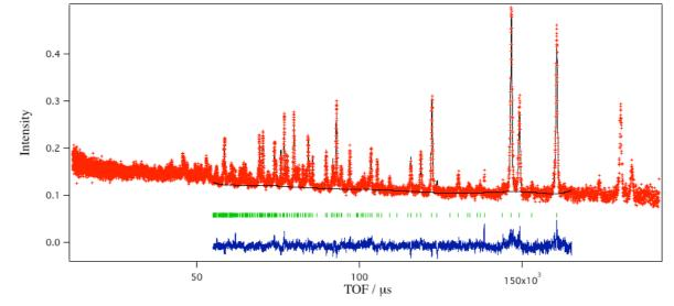
Cell parameter: a= 8.696036 Å, c= 12.620741 Å. Space group:  $P4_2/nmc$ .  $R_{\rm wp}$  = 4.25 %,  $R_{\rm p}$  = 3.54 %,  $R_{\rm e}$  = 3.20 %,  $R_{\rm B}$  = 13.06 %,  $R_{\rm F}$  = 7.25 %,  $\chi^2$  = 1.76
