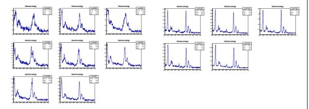
In this cycle, we observed worse energy resolution in the gamma-ray spectrum as shown above. The left figure shows the gamma-ray energy spectrum of germanium crystal located at the angle of 90 degree and the right that of the same germanium crystal in the previous measurement. We are currently improving the method to combine the data with different energy resolution.
