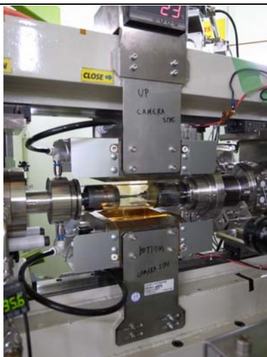
Fig. 1 The specimen mounted in a vacuum furnace on a load frame.
