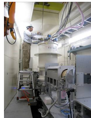
Fig. 4 The 7 T superconducting magnet on the sample table of SHARAKU.
