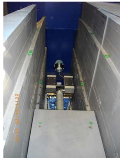
Fig.1 Installed new removable collimator
