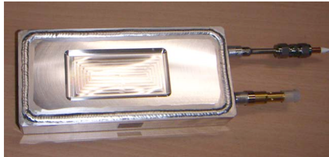
Fig. 2 The second prototype of a beam monitor.
