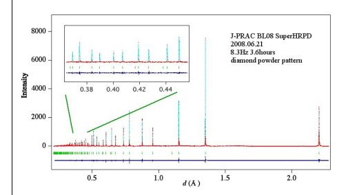
Diffraction pattern of diamond powder and its whole pattern fitting with a software *Z-Code*. *Z-Code* is a powder diffraction data analysis software suit and has been developed by us for three years. *Z-Code* composed of various kinds of programs including peak-search, peak-matching, peak-indexing, Fourier analysis, maximum entropy method, Reverse Monte Carlo, profile fitting and Rietveld method *etc*.
