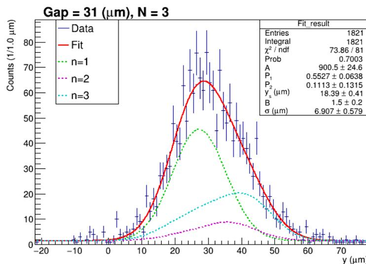
Fig. 4.12: Quantum states distribution obtained by the emulsion detector with irradiating UCN at ILL [1].
