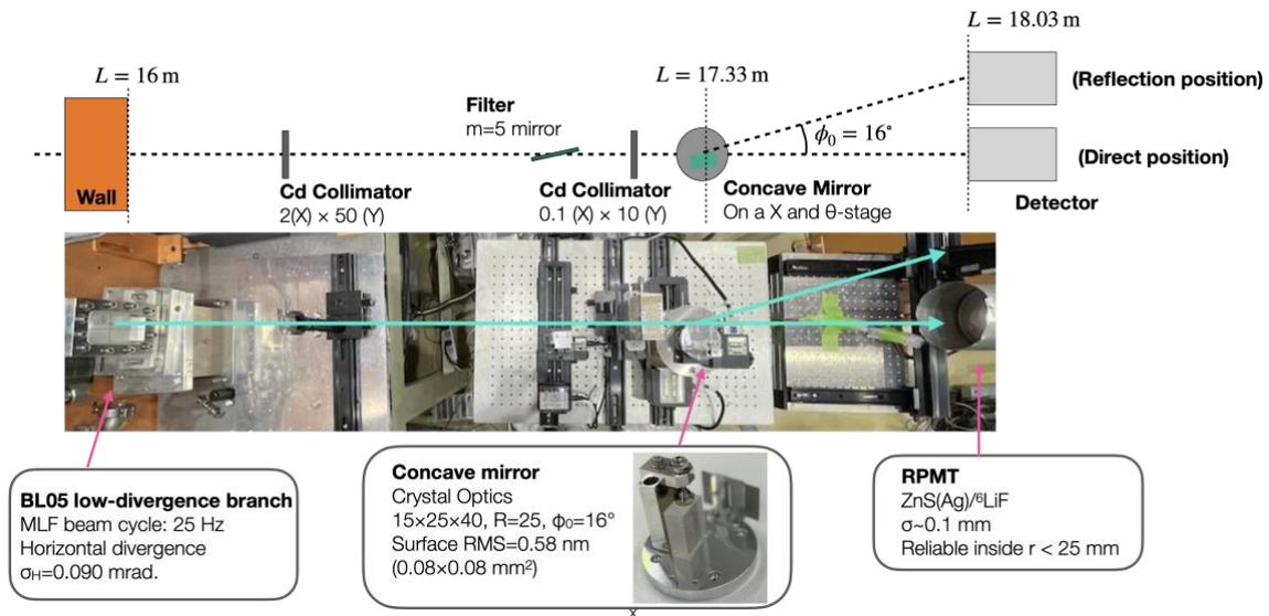
Figure 4.13: The setup of measurement of neutron whispering gallery mode at BL05 [3].
