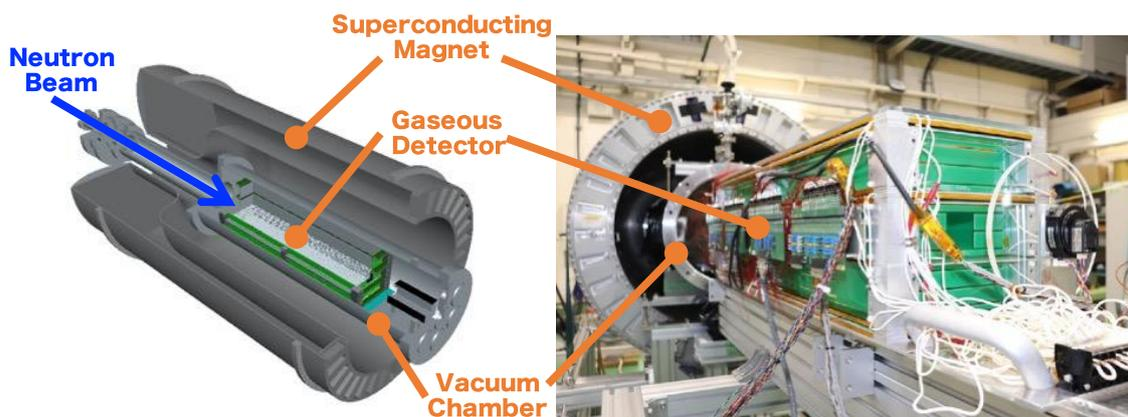
Fig 4.5: Schematic diagram (left) and photo (right) of the solenoid magnet for the LiNA experiment.
