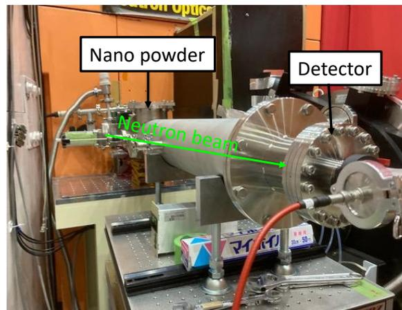
Fig. 4.11: Experimental setup for nanoparticle scattering installed in the low-divergence beam branch.
