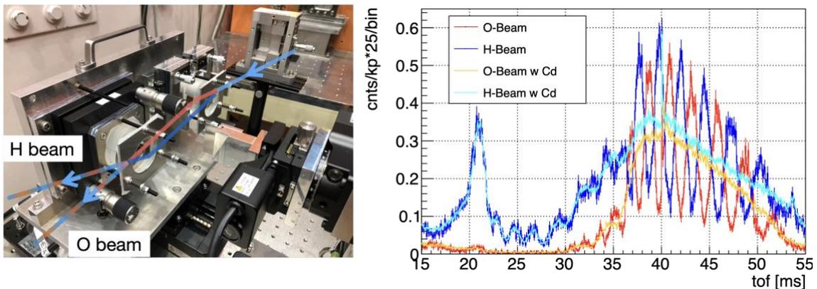
Fig. 3.4: (Left) The interferometer setup at BL05 and (Right) the measured intensities of the H and O beams. When using pulsed neutrons, interference fringes appear in TOF. The disappearance of these fringes when one path is obscured with Cd is clearly observed (orange & cyan) [3].
