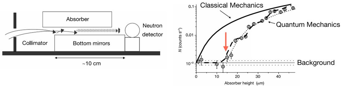
Fig. 3.7: (Left) The experimental setup where Nesvizhevsky *et al.* observed the quantization of UCNs due to gravity (right) The spectrum of UCN positions in the vertical direction [1]. The solid line represents the distribution expected from classical mechanics, and as predicted by quantum mechanics, it has been confirmed that no events occur up to the position indicated by the arrow.
