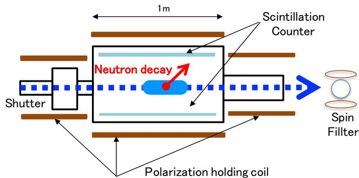
Fig. 4.6: Schematic diagram of the setup for A-term measurement. A scintillation detector for energy discrimination of decay electrons is introduced into the TPC.
