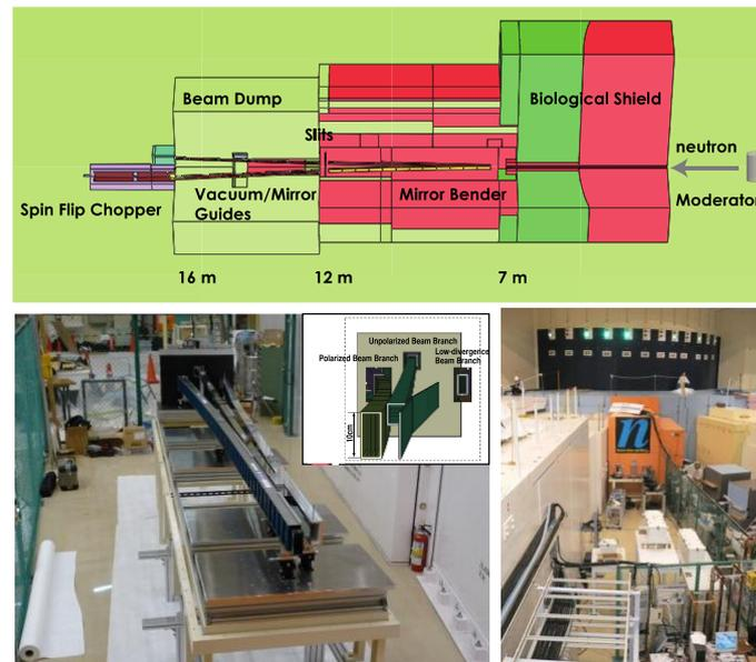
Fig. 3.1 : (Top) Schematic of BL05/NOP. (left) assembled beam benders and slits. (right) experimental area in 2010.
