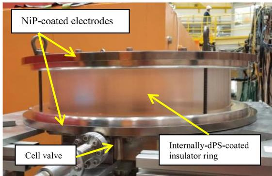
Fig. 4.10: The experimental setup for measuring the UCN accumulation time in an nEDM cell with dPS-coated plastic.
