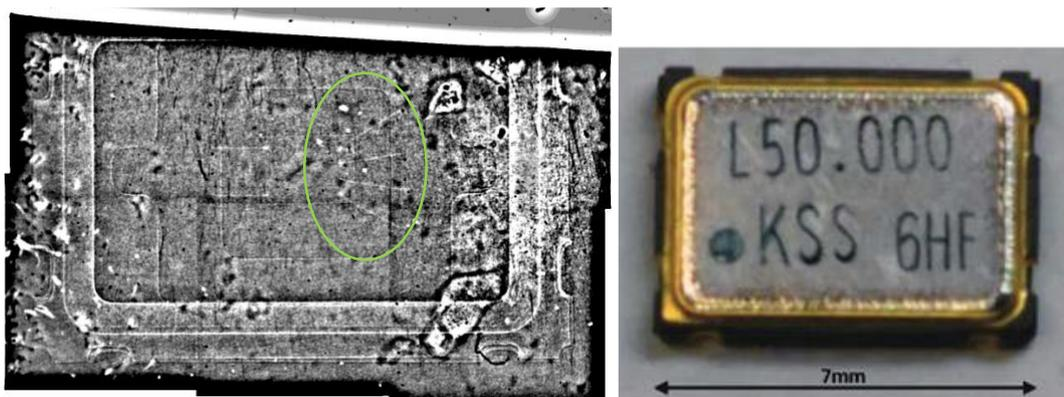
Fig. 4.14: Image of a crystal oscillator captured using a neutron emulsion detector [1]. The four gold wires can be clearly seen in the area circled in green.
