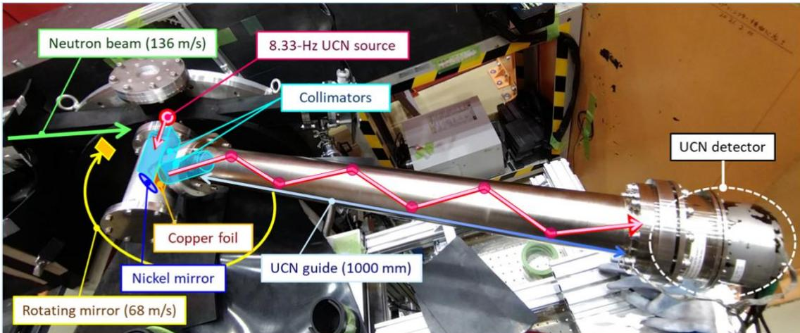
Fig. 4.9: The experimental setup for measuring the transmission/scattering rates of UCN guide tubes.
