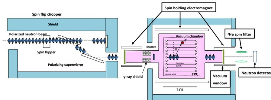
Fig. 4.3: Schematic of neutron lifetime with polarization analysis.
