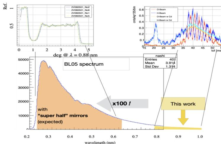
Figure 4.8: (Top left) Reflectivity of the developed supermirrors. Each  $1^\circ$  on the horizontal axis corresponds to  $m=1.2$ . (top right) currently using wavelength. (bottom center) Neutron wavelength distribution in the low-divergence beamline. It illustrates the currently used range of 0.8-1.0 nm and the range of 0.2-0.6 nm that can be covered with the supermirrors.
