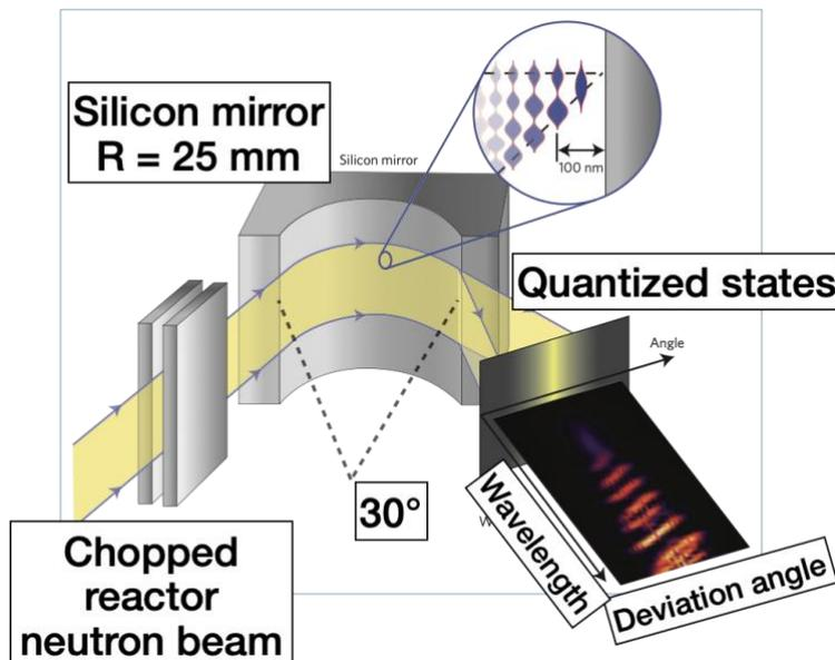
Fig. 3.9: Schematic of the neutron whispering gallery mode [6].
