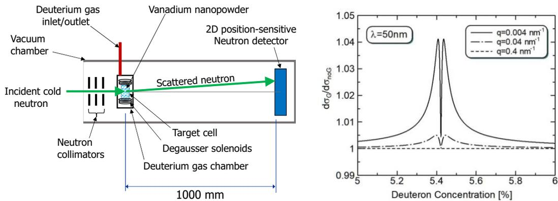
Fig. 4.12: (Left) V-D experimental setup (Right)  $q$ -dependence of scattering cross-section and D concentration.
