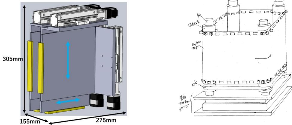
Figure 4. A side emulsion shifter (left) and an emulsion belt shifter (right).
