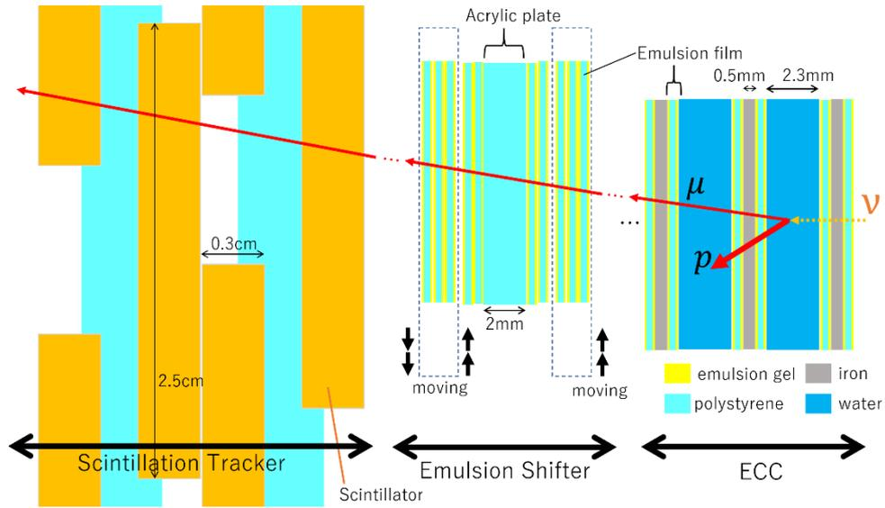
Figure 2. Detector components in the first physics run.
