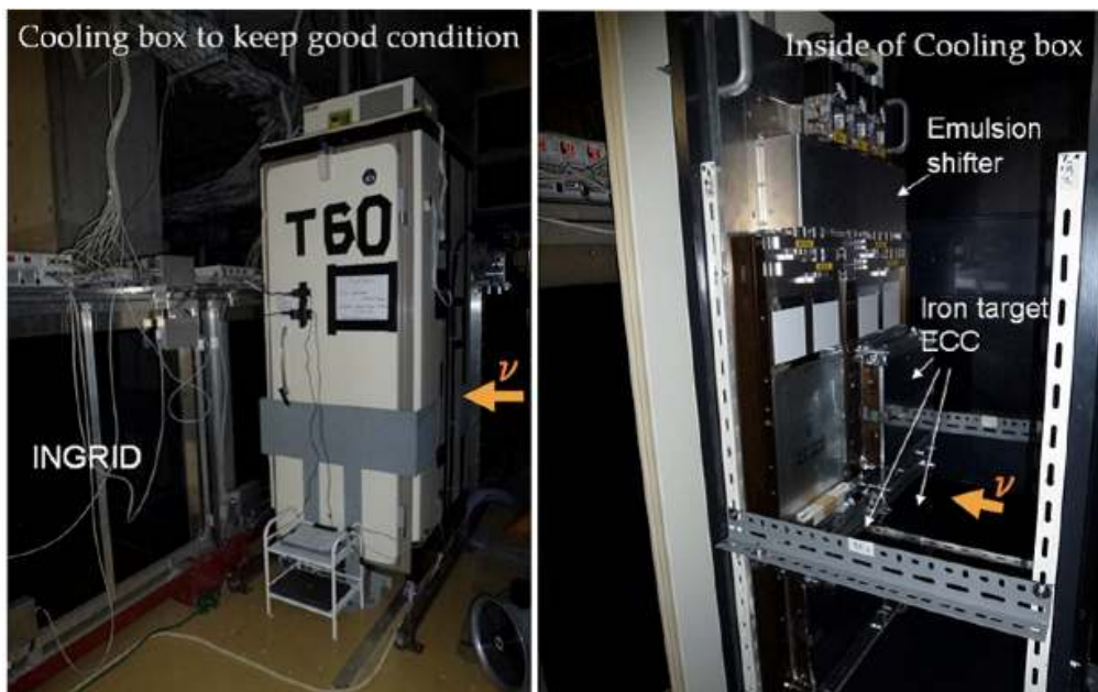
Figure 8: 60kg iron target ECC + Large emulsion shifter + INGRID
