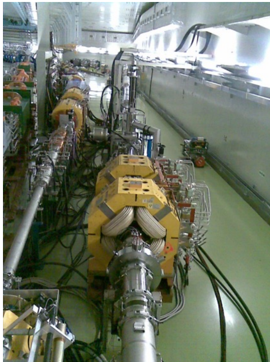
Fig. 10: Present view of candidate position 3 from upstream to downstream. Following quadrupole magnets (yellow), the chamber of the extinction monitor at candidate position 3 is shown.
