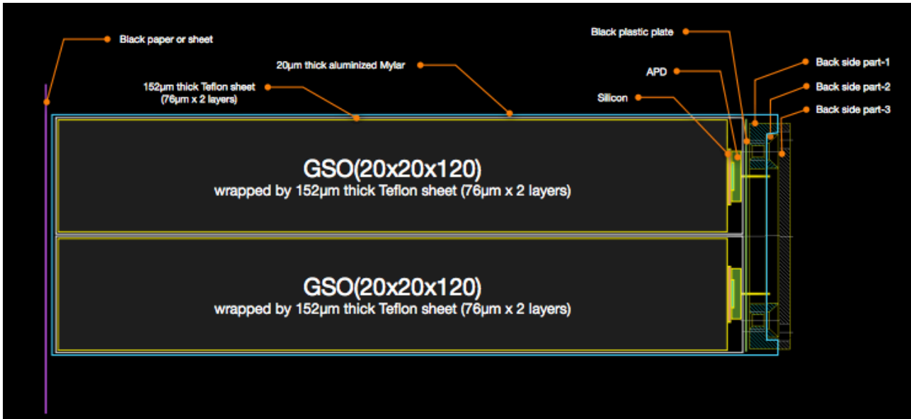
Figure 4 Schematic view of crystal and APD assembly.
