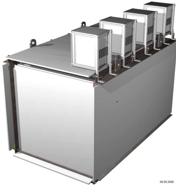
Figure 7: The detector fully assembled with veto planes and readout boxes.
