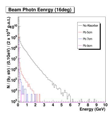
Figure 55: Beam photon spectrum with various thicknesses of Pb absorber.
