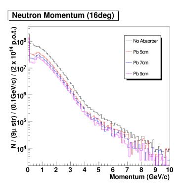
Figure 54: Neutron spectrum with various thicknesses of Pb absorber.
