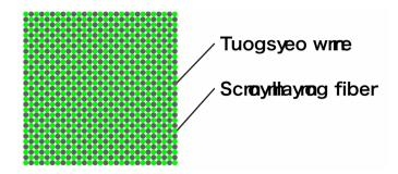
Figure 29: An option of CC03 which is made of alternating tungsten wires and scintillating fibers.
