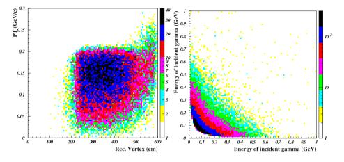
Figure 34: Left: reconstructed vertex and  $P_T$  distribution for even pairing  $K_L \to \pi^0 \pi^0$  background. It has a distribution similar to that of the  $K_L \to \pi^0 \nu \overline{\nu}$  decay. Right: Energy distribution of gammas that enter the veto counters. At least one photon has sufficiently high energy to trigger the counter with a high detection efficiency.
