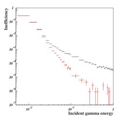
Figure 25: Comparison of the  $\gamma$ -detection inefficiency of the Main Barrel between E391a and Step 1. In Step 1, we will add additional modules made of 5 layers of alternating 5-mm-thick lead and 5-mm-thick scintillation plates. Black points are the inefficiency of the E391a Main Barrel, and red ones are for Step 1.
