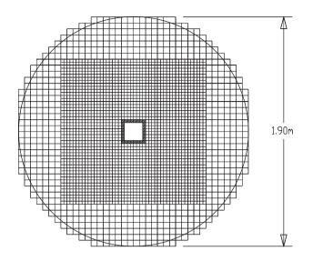
Figure 15: Layout of the Calorimeter for the J-PARC experiment with the KTeV CsI crystals. The  $2.5 \times 2.5 \times 50$ -cm<sup>3</sup> crystals are used for the inner region, and  $5.0 \times 5.0 \times 50$ -cm<sup>3</sup> crystals are used for the outer region.
