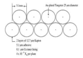
Figure 51: Design of vacuum straw tubes.
