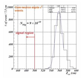
Figure 44: Reconstructed vertex for the  $\pi^0$  events produced at the Charged Veto. In E391a, the background level is estimated to be ~  $9 \times 10^{-10}$  for the experiment with a single event sensitivity of  $9 \times 10^{-8}$ . The  $\pi^0$  background from Charged Veto is still negligible in Step 1 with  $10^{-12}$  sensitivity.
