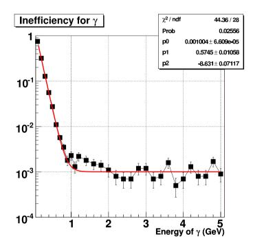
Figure 58: Expected photon inefficiency of the BHPV. We require three or more consecutive hits along the beam direction, where the threshold of each module is set to be 4 photoelectrons. In the calculation, photons are injected randomly in a region of 15-cm diameter and normal to the BHPV face. The red curve indicates our inefficiency function Inefficiency  $= p0 + \exp(p1 + p2 * E_{\gamma})$ , which is used later for background estimations.
