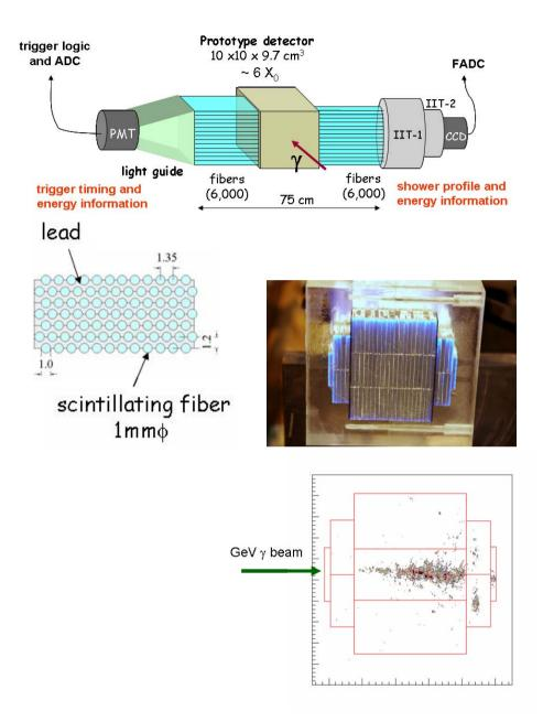
Figure 50: Prototype of the spaghetti calorimeter (top); fiber alignment in lead (middle left); cross section of the prototype (middle right) and shower development of 1-GeV photons recorded in the beam test (bottom).
