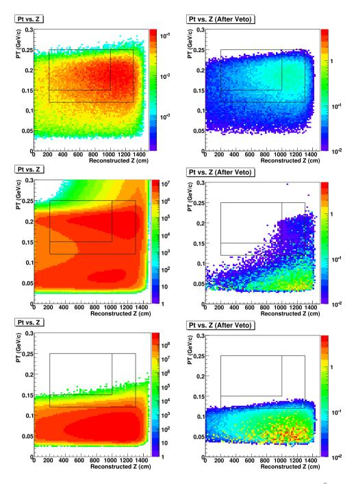
Figure 48: Distributions of  $P_T$  vs. the reconstructed Z position for  $K_L^0 \rightarrow \pi^0 \nu \overline{\nu}$  signal events (top),  $K_L^0 \rightarrow \pi^0 \pi^0$  (middle) and  $K_L^0 \rightarrow \pi^0 \pi^+ \pi^-$  (bottom) background events before (left) and after (right) imposing the photon veto cuts, respectively.
