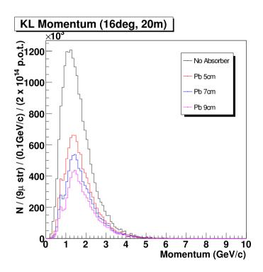
Figure 53:  $K_L$  spectrum with various thicknesses of Pb absorber.
