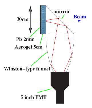
Figure 30: Schematic view of the BHPV module.
