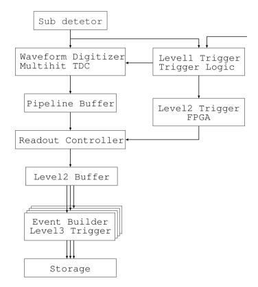
Figure 32: Schematics of data acquisition system
