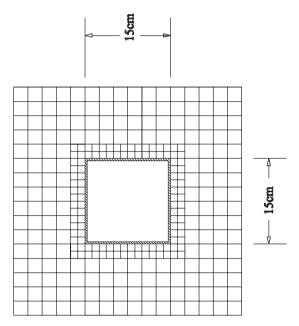
Figure 19: Layout of the CsI around the beam-hole region of the Calorimeter. In this configuration, the inner-most 2.5-cm layer consists of  $1.25 \times 1.25 \times 50.0$ -cm<sup>3</sup> PbWO<sub>4</sub> crystals, a total of 112 blocks. The square carbon fiber pipe is 4 mm thick.
