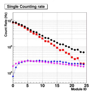
Figure 61: Estimated BHPV counting rates as a function of module ID, where ID 0 (24) means the most upstream (downstream) module. The detection threshold is set to be 4 photoelectrons. The square, triangle, and inverted triangle points show the contributions from beam photons, neutrons, and  $K_L$ 's, respectively, and the circle points indicate their sum.
