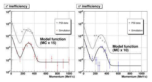
Figure 57: Inefficiencies for negative (left) and positive pions (right), with the combination of charged particle detectors and photon counters behind them. The shape of the curve is obtained by fitting the simulation result, as indicated by the lower curve in the plots. We scaled it to reproduce the measured data by the PSI group, as indicated with dashed line, and used it as the model function of pion inefficiency.
