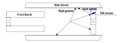
Figure 23: Schematic view of a shower back-splash.
