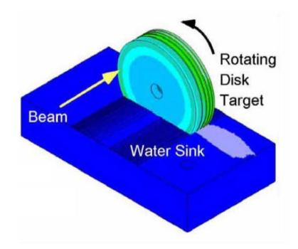
Figure 52: Schematic drawing of the T1 target, prepared by the J-PARC Target Monitor Group.
