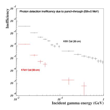
Figure 17: Photon detection inefficiency of the Calorimeter due to punchthrough. In the KTeV CsI crystals, the inefficiency is negligible compared to that due to photonuclear interactions, while these inefficiencies are comparable in the E391a CsI crystals.
