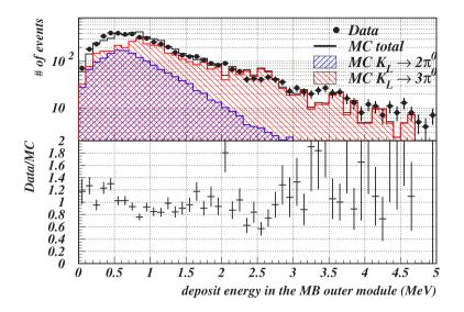
Figure 22: Top: The distribution of the energy deposit in the Main Barrel for the data (dots) and Monte Carlo (M.C.) results to  $K_L \to \pi^0 \pi^0$  decay (blue hatched) and  $K_L \to \pi^0 \pi^0 \pi^0$  decay (red hatched). Bottom: Ratio of the data to M.C.
