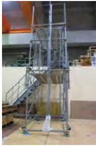
mock-up scaffolding (4.5 m high)
