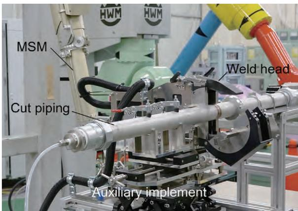
Fig. 9. Photo of the release procedure of the weld head after welding.
