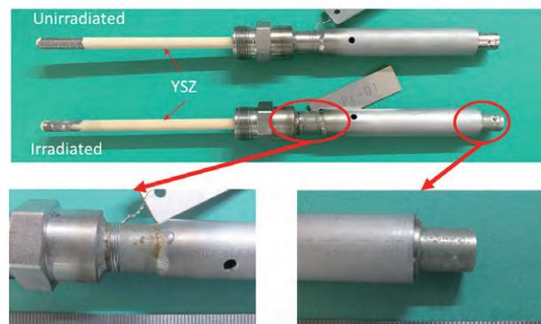
Fig. 7. Oxygen sensors before (upper) and after irradiation (lower) by gamma-rays.
