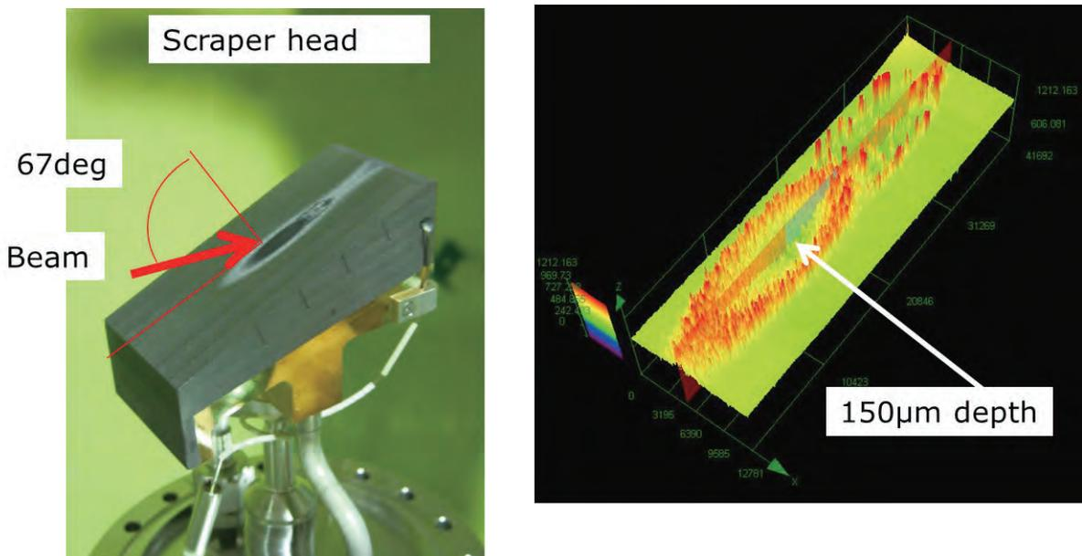
Fig. 6. Observation of scraper surface after 9 months operation.
