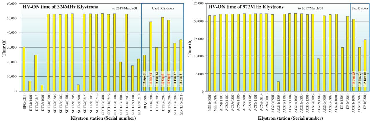
Fig. 7. Operating time of 324-MHz (left) and 972-MHz klystron (right) as of March 2017.
