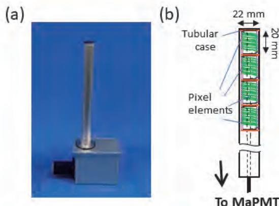
**Fig. 4.** A 14-element prototype detector. (a) Photograph and (b) a schematic view of the detector
