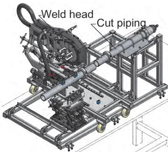
Fig. 8. Sketch of the prototype of the auxiliary implement.
