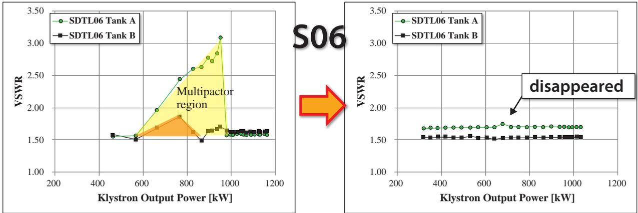
Fig. 5. VSWR as a function of the klystron output power at S06 before (left) and after (right) surface cleaning.
