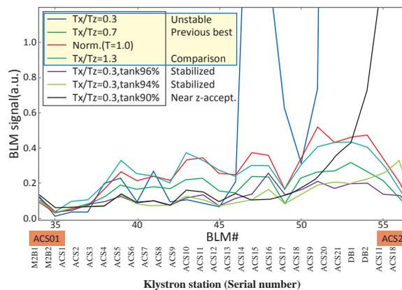
Fig. 8. Measured beam loss at beam loss monitors for the transverse and longitudinal redesigning for the J-PARC linac ACS section.
