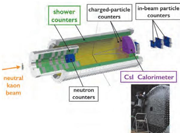
**Fig. 6.** Schematic drawing of the detector for the KOTO experiment.
