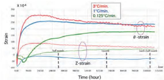
Fig. 10. Strain behavior for the samples under various cooling conditions.
