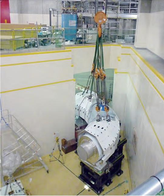
**Fig. 5.** Alignment of the muon transport solenoid.
