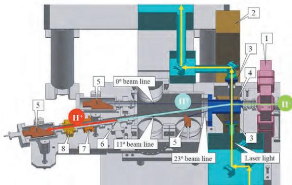
**Fig. 12.** Schematic view of the LCE system (1- quadrupole magnet, 2- bending magnet, 3- quartz viewing port, 4- vacuum chamber, 5- beam dump, 6- stripping foil, 7- beam position monitor, 8- slow current transformer).
