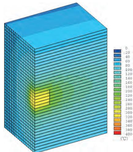
**Fig. 4.** Temperature distribution of the core in the acceptable case.
