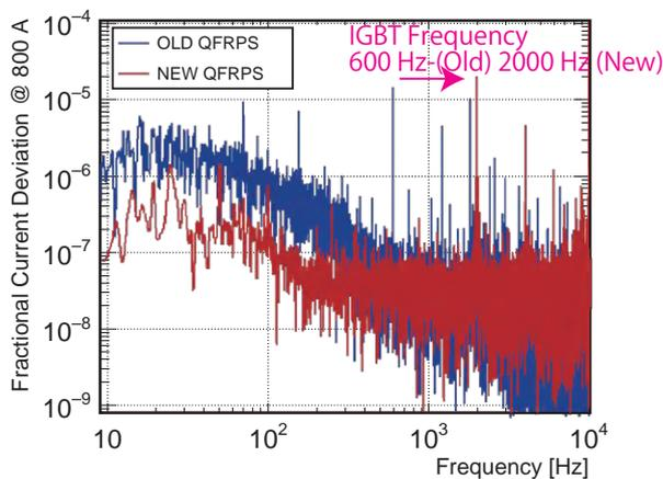
**Fig. 13.** Spectrums of the current ripple. Blue: Old power supply, Red: New one. Data was taken at the flat top of SX-mode pattern.
