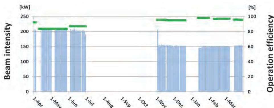
**Fig. 1.** Target operation history in JFY2016. The blue histogram indicates the incident proton beam intensity and the green lines represent the average operation efficiency in each accelerator run cycle.
