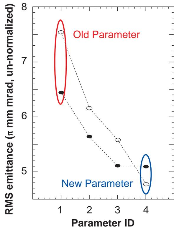
Fig. 11. Extraction beam emittance measurement results.
