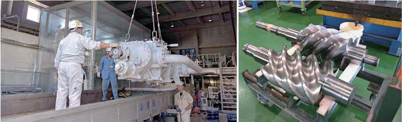
**Fig. 3.** Picture of the screw compressor to be overhauled (left), and the screws at the inspection (right).
