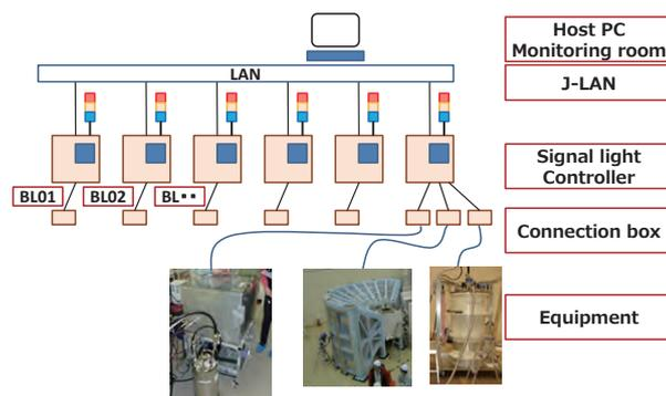
Fig. 6. Schematic of the alarm indication system.
