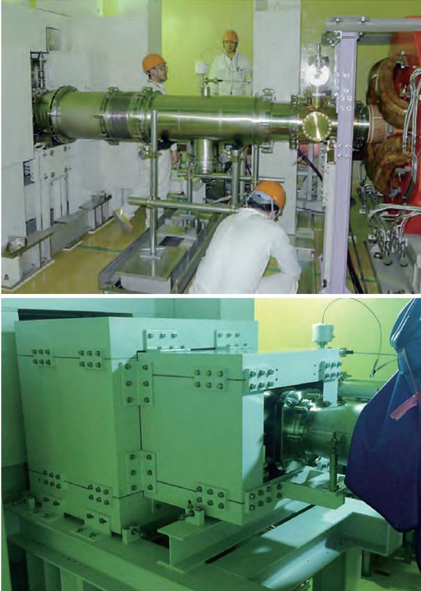
Fig. 9. Temporary spare duct and new collimator.
