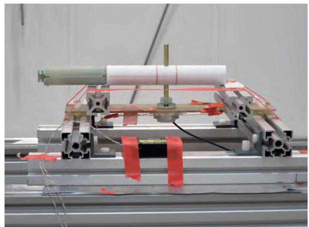
**Fig. 6.** Material effect measurement of a new standard probe in ANL.
