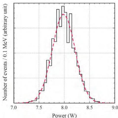
**Fig. 13.** Power distribution of the charge-exchanged  $\text{H}^+$  beam. Here, the value of the horizontal axis represents the converted power under the J-PARC linac beam condition.
