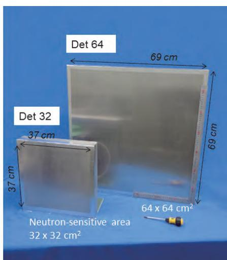
**Fig. 3.** Prototype detectors with neutron-sensitive areas of  $32 \times 32$  and  $64 \times 64$  cm<sup>2</sup> (Det 32 and Det 64) [1].
