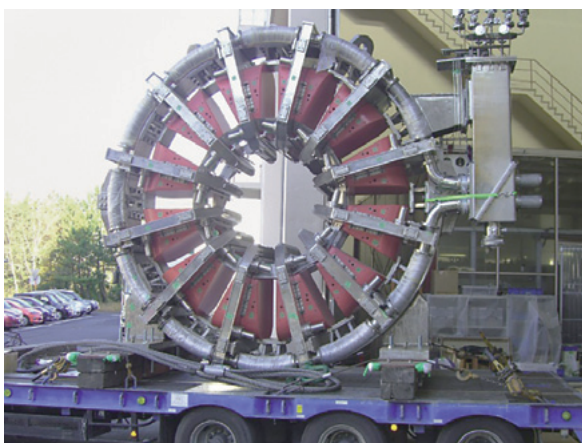
Fig. 5. Transportation of the superconducting toroidal magnet (left) and the system installation work (right).
