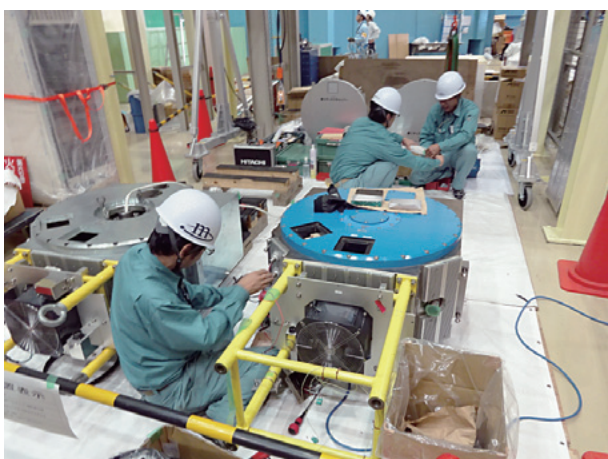
Fig. 10. Maintenance of BL01 T0 chopper
