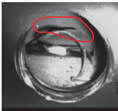
Fig. 2. Disk-shaped specimen cut out from the target vessel. The mercury flow facing surface of the specimen is outlined with red line.
