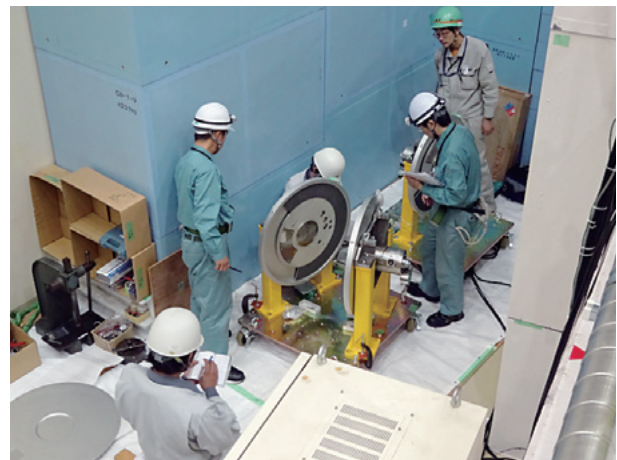
Fig. 9. Maintenance of BL15 low-speed disk chopper.
