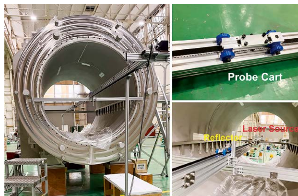
Fig. 6. Setup for measuring the magnetic field of the DS using position calibration with a laser tracker
