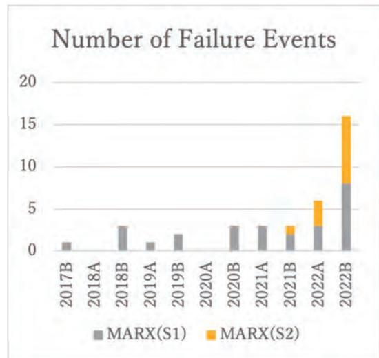
**Fig. 7.** Number of MARX board failures that occurred in each operating period. Gray (yellow) bars represent the number of failures in the circuit that kicks the beam toward S1 (S2), respectively.
