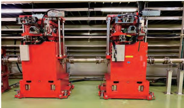
**Fig. 18.** Collimator C (left) and D (right, installed in 2022) in insertion A.
