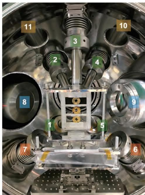
**Fig. 4.** Picture of the Hemispheric chamber in the view from downstream of the beam. Gold coins are set at a sample position. The Ge detectors and multi-pixel detectors are equipped at Port 1 - 7, and Port 8 - 9, respectively. Ports 10 -11 can be used for decay counters and other detectors.
