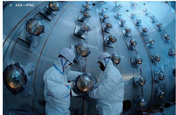
**Fig. 3.** PPMT installation in the new JSNS<sup>2</sup> detector.
