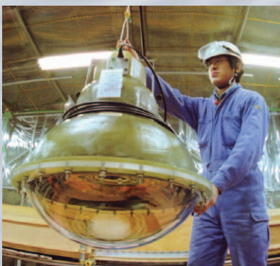
A photomultiplier tube used in Super-Kamiokande. The diameter is 50 cm — the world's largest.
